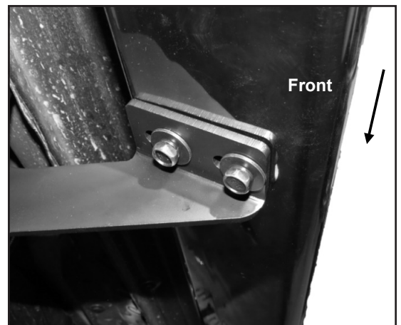
(Figure 11) Passenger/Right Main Tube attached to Mounting Bracket.
